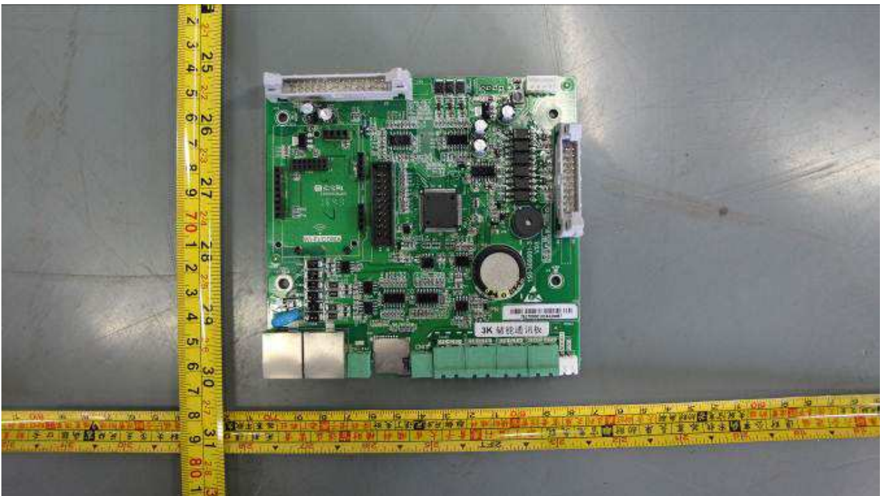
Communication board view
